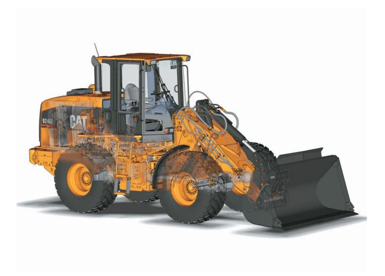
**Caterpillar Engine**. The six-cylinder 3056E Direct Injection Turbocharged (DIT) engine with Air-to-Air After Cooler (ATAAC) has a proven reputation for reliability, durability and performance. Fuel injection is electronically controlled for precise timing.
