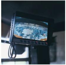
**Optional Rear View Camera System.** Work area visual enhancement system utilizes a closed circuit video monitoring system. One, two or three cameras can be mounted on the machine frame. Objects can be viewed in a 7 inch color LCD monitor located in place of the right cab rear view mirror. Rear view system is compatible with heavy duty radiator guarding and waste handling packages.
