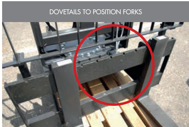
EQUIPPED WITH ROTATION BLOCKING BAR +/- 90°
