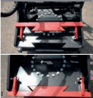
EQUIPPED WITH ROTATION BLOCKING BAR +/- 90°
