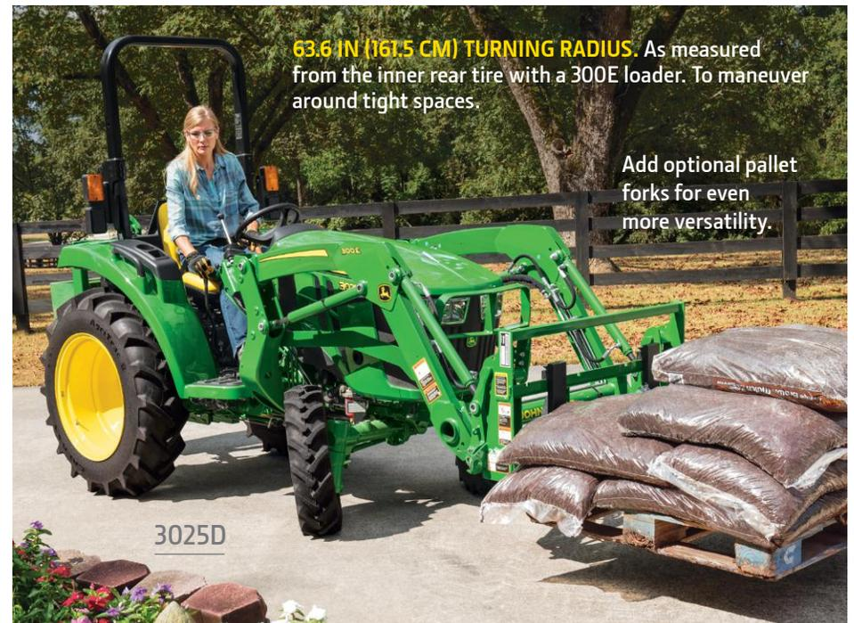
**63.6 IN (161.5 CM) TURNING RADIUS.** As measured from the inner rear tire with a 300E loader. To maneuver around tight spaces.
