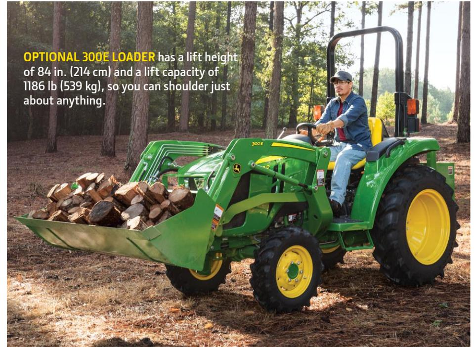
**OPTIONAL 300E LOADER** has a lift height of 84 in. (214 cm) and a lift capacity of 1186 lb (539 kg), so you can shoulder just about anything.
