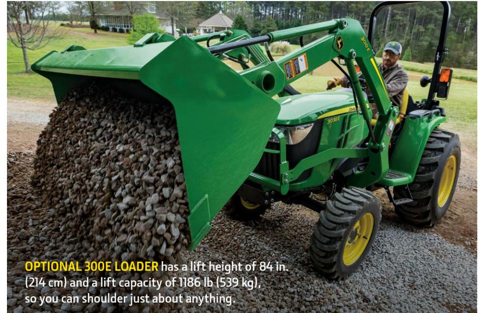
**OPTIONAL 300E LOADER** has a lift height of 84 in. (214 cm) and a lift capacity of 1186 lb (539 kg), so you can shoulder just about anything.
